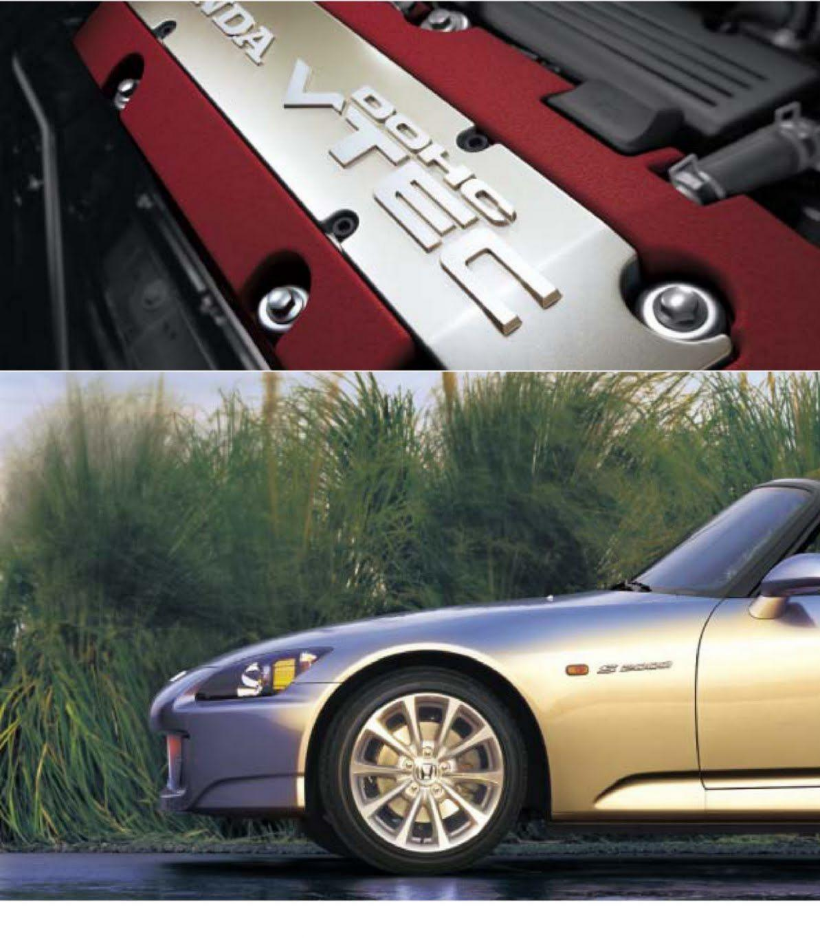
Honda's revolutionary Variable valve Timing and lift Electronic Control (VTEC®) technology overcomes a long-time limitation of traditional engine design. With VTEC, no compromises have to be made between low-rpm and high-rpm performance. One cam lobe is tuned for low-end torque. At higher revs, another lobe takes over valve operation for a boost in high-end horsepower. So whatever the engine speed, power and efficiency are always optimal.
